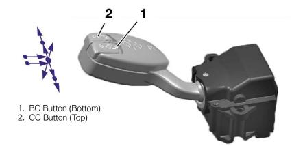
The CC button in the turn signal stalk can be used to browse through all the CC messages issued (press briefly), or to toggle between the On-Board Computer and Check Control in the display area below the tachometer.
